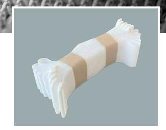
The Ring Straps (standard white) are made from woven polyamide. A large portion of the loop strap is connected to a smaller portion of the hook strap using ultrasonic welding. The end of the hook section is equipped with an "easy peel," which means that the closure can be easily opened. By threading the hook section through the buckle and then pressing it onto the loop strap, you achieve a reliable and secure closure that is easy to adjust.
