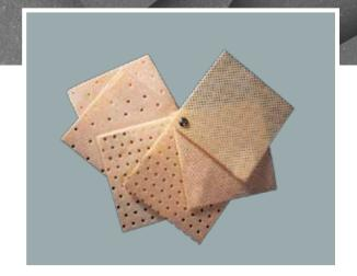
The White Label One Side Coated thermoplastic material is a low-temperature thermoplastic material resulting from copolymerization based on polycaprolactone and polyurethane, coated on one side with a foam layer of 0.6 mm thickness. This unique foam layer creates an air layer between the patient's skin and the thermoplastic.
